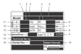
Fig. 11 Nameplate of CRFlex pump end
