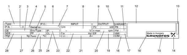
Fig. 1 Nameplate of the MGFlex motor
