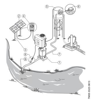
Fig. 15 CRFlex Solar with level switch
