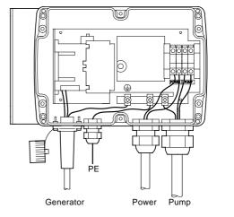
Fig. 9 Electrical connections, IO 101
