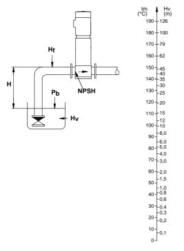
Fig. 12 Minimum inlet pressure - NPSH
