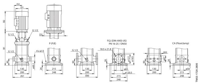
Fig. 23 Dimensional drawing sketch of CRIF/CRNF 15-1
